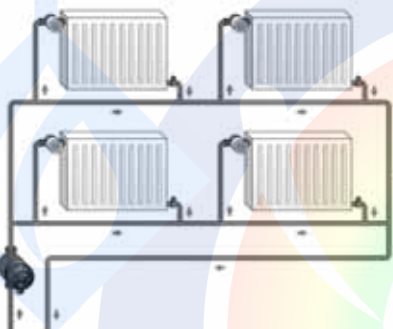
Fig. 1 One-pipe heating system
