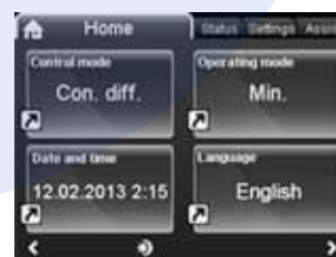
Fig. 1 Example of main display on a TPE Series 2000 with advanced control panel
