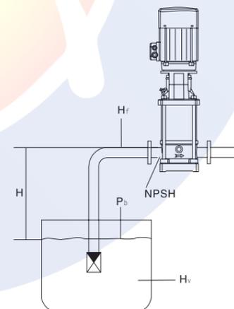
**Note:** To avoid cavitation, never select a pump with a duty point too far to the right on the NPSH curve. Always check the NPSH value of the pump at the highest possible flow.
