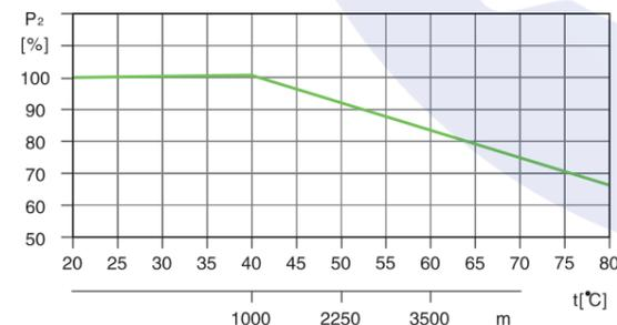
For example, when the pump is installed at altitude of more than 3500 meters above sea level, P<sub>2</sub> will be decreased to 88%. When the ambient temperature is 70°C, P<sub>2</sub> will be decreased to 78%.
